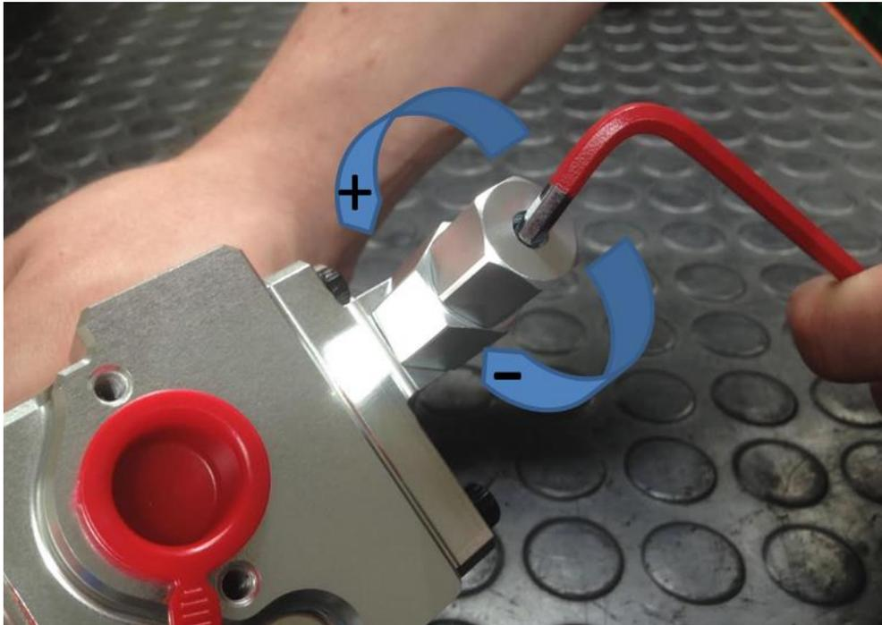
USING A 4MM ALLEN KEY, ADJUSTMENT OF THE PRV IS AS FOLLOWS:
